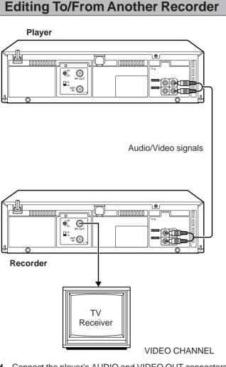
1 Connect the player's AUDIO and VIDEO OUT connectors to the recorder's AUDIO and VIDEO IN connectors.
